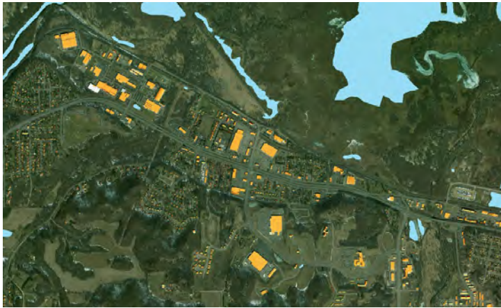
FIGURE 3.10 RED WING'S ROOFTOP SOLAR RESOURCE POTENTIAL
