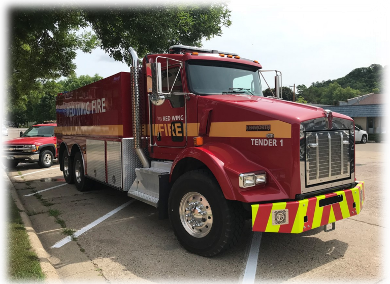
Tender 1 – 2014 Danko 3500 Gallon Water Tank 400 GPM Pump
