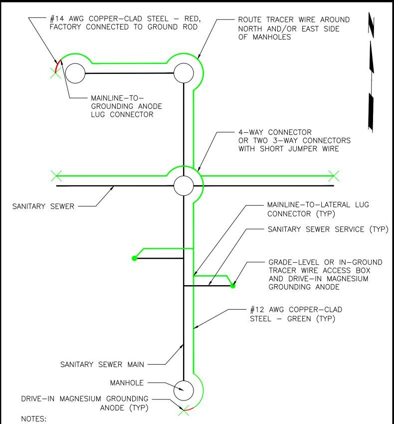
1) TRACER WIRE SHOWN AWAY FROM PIPE FOR CLARITY. WIRES SHALL BE INSTALLED ON THE BOTTOM SIDE OF THE PIPE BELOW THE SPRING LINE. THE WIRE SHALL BE FASTENED TO THE PIPE WITH TAPE OR PLASTIC TIES AT 5' INTERVALS.
