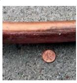
Copper Scratch Test: The scratched area is copper color, like a penny.
