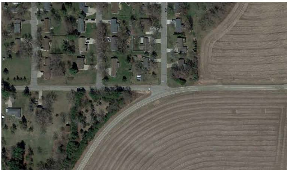
Exhibit 3: Skewed Intersection Example (Spring Creek Road at Mill Road) – Google Earth Aerial
